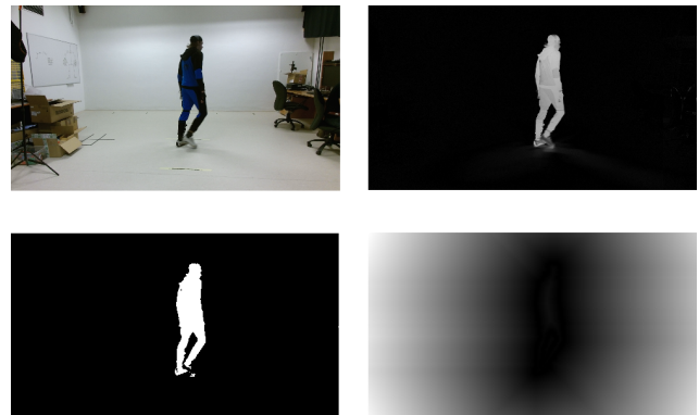
Figure 5: Tracking of the actor position using Chamfer matching. (Top) an input image and the subtracted background image in grayscale. (Bottom) applied adaptive thresholding and calculated distance transform of the silhouette.
