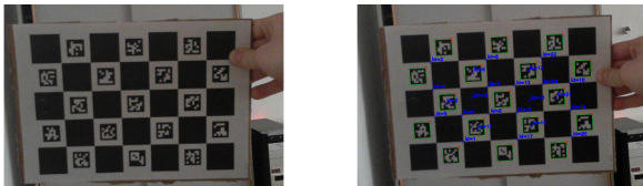
Figure 1: The ChArUco calibration board. The ChArUco is a combination of the classical calibration checkerboard and the ChArUco alphabet signs.
