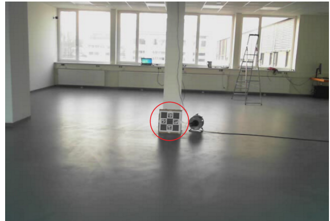
Figure 2: A model-view matrix that consists of a rotation and a translation of the ChArUco board into the camera image is obtained in the tracking start-up phase. Thus, the origin of the virtual scene is set into the ChArUco board location and the camera position and orientation are set accordingly.
