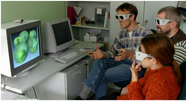
Figure 3: Conventional desktop VR with an active stereo system.
