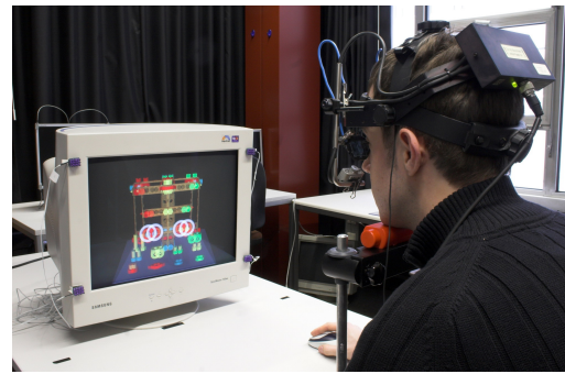
Figure 4: The set-up of the experiment used shutter-glasses and a cathode-ray display. The head of the user was stabilized using a chin rest.
