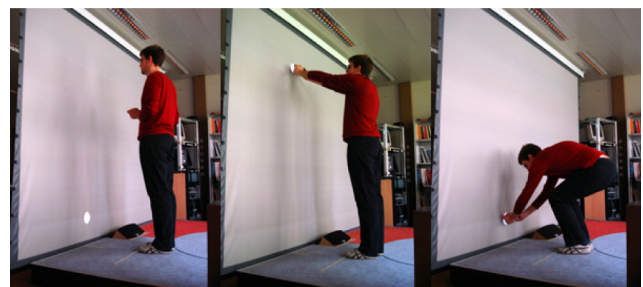
Figure 4: Experimental setup for the study in the real world. The subject is at a distance H/3 from the screen and must reach targets at height going from 0.2H to 1.1H . H being the subject height.
