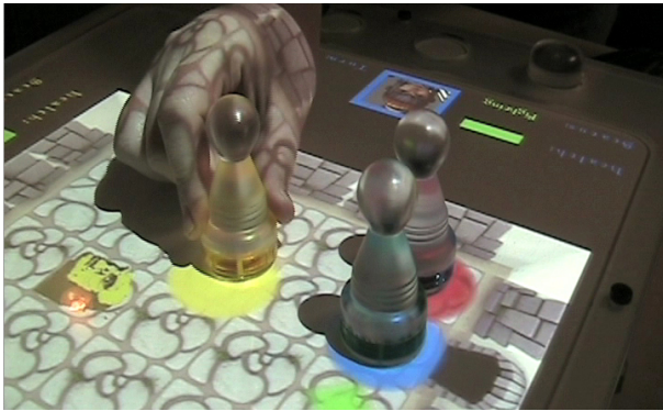
Figure 4: Players use tagged physical pawns to move their characters around the virtual space
