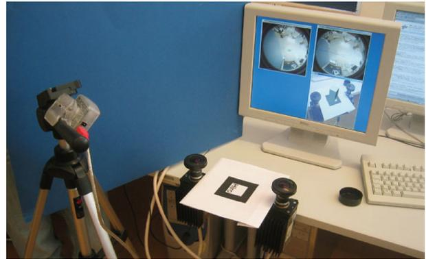
Figure 1: Webcam, HDR-cameras with marker, augmented scene on display
